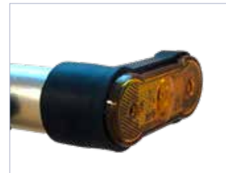
Example in which the side marker light is mounted on a rubber bracket
